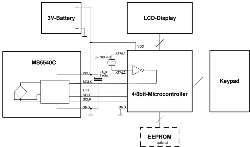
Figure 7: Demonstration of MS5540C in a mobile altimeter
