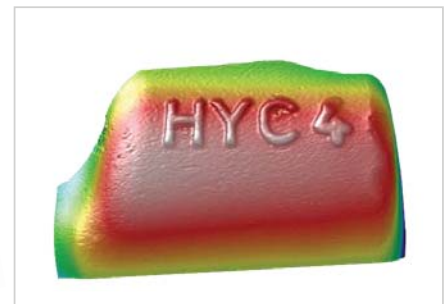
3D text recognition of embossments which cannot be solved with 2D image processing due to lack of contrast
