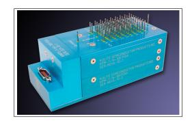
The KMPS-1-64 is a 64 position pressure scanner with both high accuracy digital and analog outputs. This allows it to be used with both legacy analog systems and new digital systems. The RS-485 digital output allows multiple scanners to be read over a single data bus. The ethernet digital output allows integration into standard networks using TCP or UDP. The KMPS also features purge and auto-zero capabilities.
