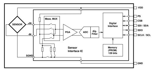
Figure 1: Block diagram of MS5803-30BA
