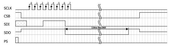
Figure 9: Reset command sequence SPI (mode 0)
