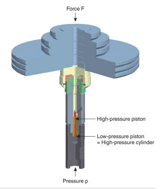
Dual-range piston-cylinder system 2,600 bar
