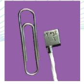
An Ultra-lightweight miniature triaxial vibration transducer comprising of three voltage output piezo-electric accelerometer elements mounted orthogonally within a titanium block. It makes use of the independent shear plate sensing elements, ensuring a rugged and repeatable triaxial measurement under the most extreme conditions. This design will outperform single element devices. The AT/08 uses high temperature piezo-ceramics as standard to ensure thermal stability.
