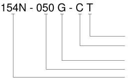
Vent (T = Tube, Blank = No Tube) Electrical (C = Ribbon Cable with Connector, R = Ribbon Cable, P = Solder Pads) Type (A = Absolute, G = Gage) Pressure Range Model
