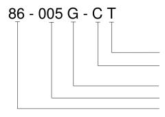
Vent (T = Tube, Blank = No Tube) Electrical (C = Ribbon Cable with Connector, R = Ribbon Cable, P = Solder Pads) Type (A = Absolute, G = Gage) Pressure Range Model
