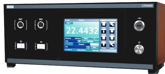
Multi-functional precision thermometer, model CTR4000
