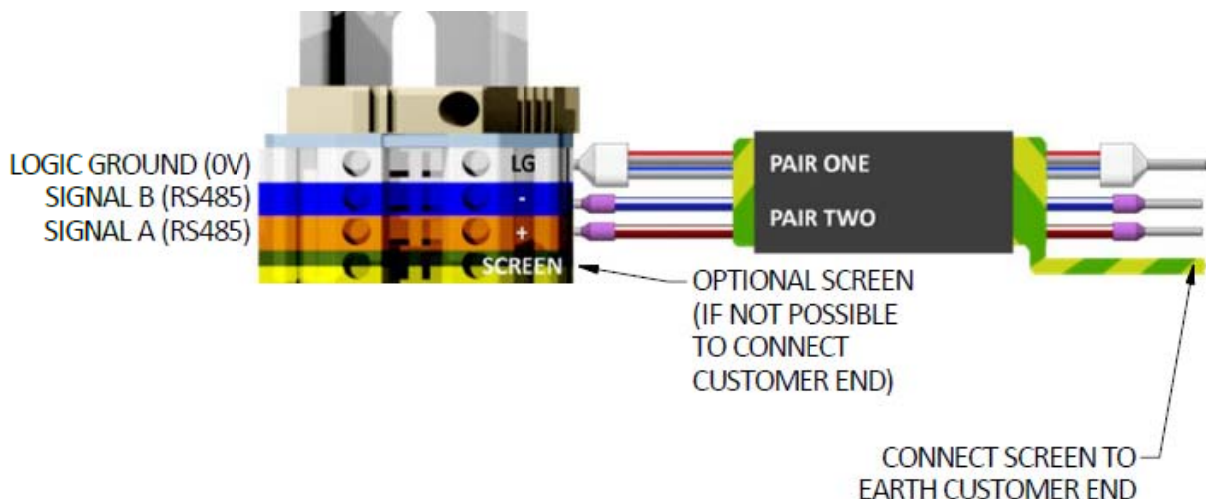
Wiring Diagram 2 – Modbus
