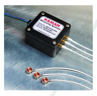
In many applications the actual motion to be monitored can be very small. A full scale calibration of 100 microns is not unusual, and with a full scale output of 10VDC, sensitivity is high, in this case 100mV/micron.
