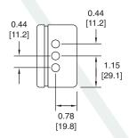
Note: Single channel units use center connector, dual channel units use top and bottom connectors.
