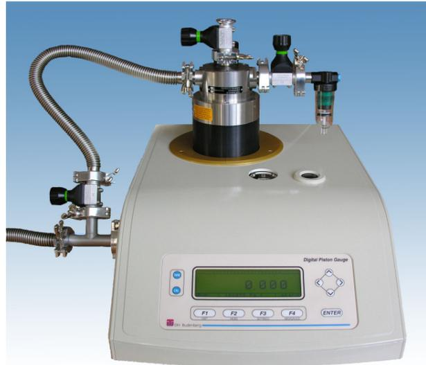
CPD8000-A fitted with low pressure head
