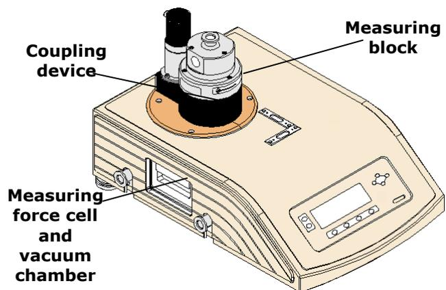
The measuring force cell is associated with an Auto Calibrating Function (see further) which enables to apply to it, easily and whenever it is necessary, a reference force that is equivalent to the product of the mass multiplied by the local acceleration of the gravity ( $F = M \times g$ ) in order to recalibrate it.
