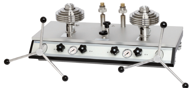
Model CPB5600DP pressure balance for differential pressure
