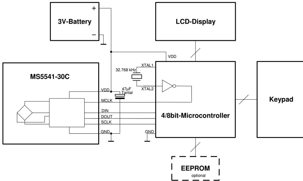
Figure 7: Demonstration of MS5541-30C in a diving computer
