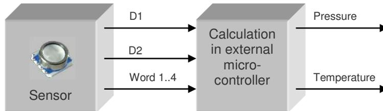
For both pressure and temperature measurement the same ADC is used (sigma delta converter):
