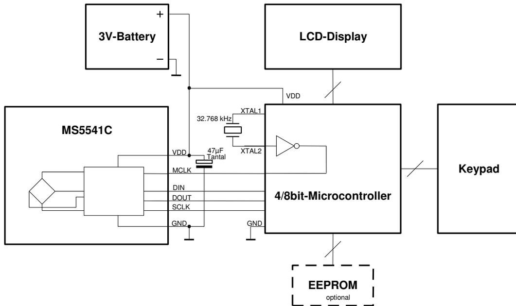
Figure 7: Demonstration of MS5541C in a diving computer
